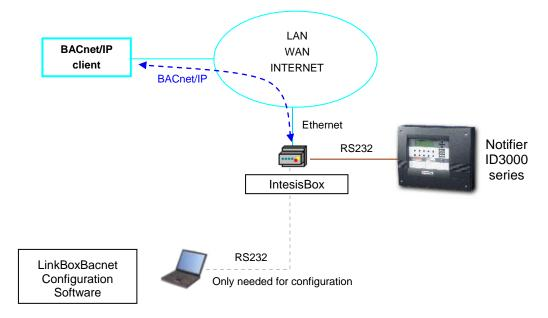
Monitor & Control your network of Notifier fire panels remotely from your Control Center using any commercial SCADA or monitoring software with BACnet/IP driver.
