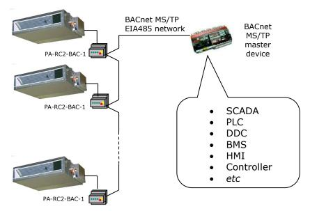
The PA-RC2-BAC-1 interface allows a complete and natural integration of **Panasonic** air conditioners into either BACnet IP or MS/TP networks. Compatible with the ECOi and PACi line models commercialized by PANASONIC
