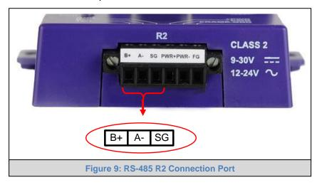
Connect to the 3 pins on the left-hand-side of the 6 pin connector as shown.
