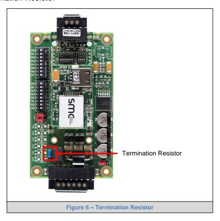
Termination resistors are also used to reduce noise. These pull the two lines of an idle bus together. However, they would override the effect of any bias resistors, if connected.
