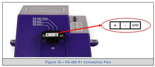
The following Baud Rates are supported on the R1 Port:
