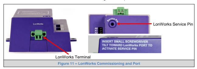
To commission the QuickServer LonWorks port, insert a small screwdriver in the commissioning hole on the face of the QuickServer's enclosure to access the Service Pin. See the instructions on the QuickServer as to which way to toggle the screwdriver during commissioning.
