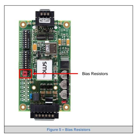
The QuickServer bias resistors are used to keep the RS-485 bus to a known state, when there is no transmission on the line (bus is idling), to help prevent false bits of data from being detected. The bias resistors typically pull one line high and the other low - i.e. far away from the decision point of the logic.
