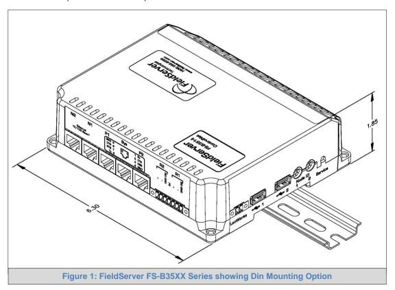
**NOTE:** Install only as instructed, failure to follow the installation guidelines or using screws without the DIN Rail Mounting Bracket could result in permanent damage to the product.
