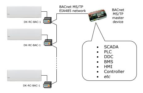
The DK-RC-BAC-1 interface allows a complete and natural integration of *Daikin* air conditioners into either BACnet IP or MS/TP networks. Compatible with SKY & VRV air conditioner lines commercialized by Daikin.
