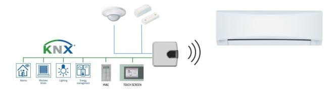
IntesisBox® IS-IR-KNX-1i allows monitoring and control of Air Conditioners from KNX installations. Compatible with most AC units with an IR receiver (check section 3 for more information).
