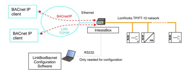
IntesisBox is a BACnet/IP Server device allowing read/write network variables (SNVTs) of LON devices connected to a LON network, and offering these values through standard BACnet objects. SNVT values in LON can be read/write from BACnet. Each LON basic data type of network variables in LON devices can be mapped into an individual BACnet object.
