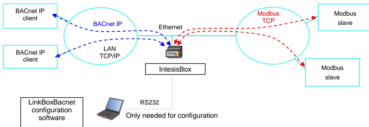
**Figure 1.1** Integration of Modbus TCP and BACnet/IP using *IntesisBox BACnet/IP Server - Modbus TCP Master* gateway
