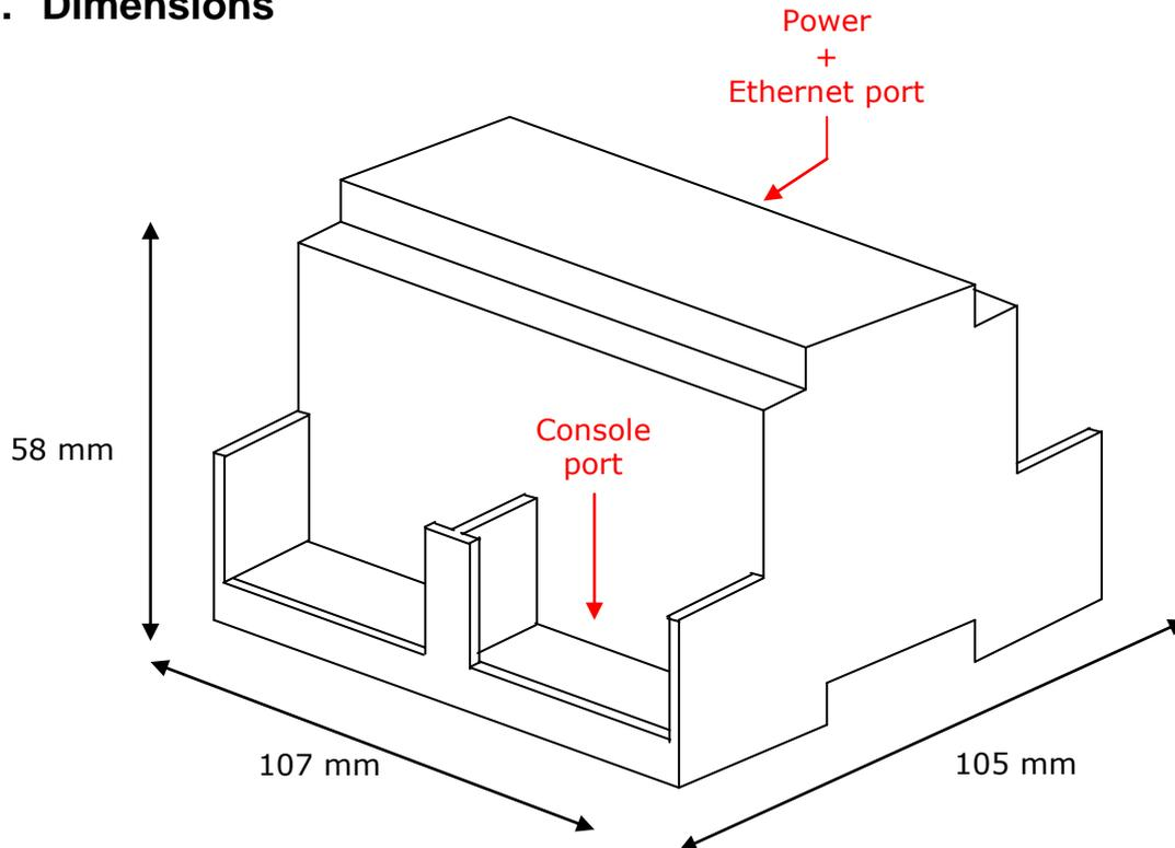
Free space recommended to install the device into a cabinet (wall or DIN rail mounting), with space enough for external connections:
