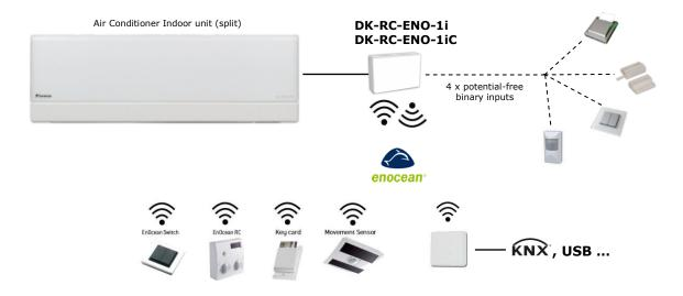
IntesisBox<sup>®</sup> DK-RC-ENO-1i allows monitoring and control, fully bi-directionally, all the functioning parameters of DAIKIN Air Conditioners from EnOcean installations.
