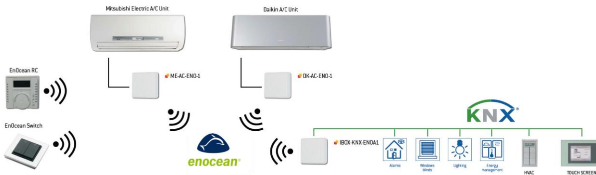
Figure 4.1 IBOX-KNX-ENO-A1 / A1C integration example
