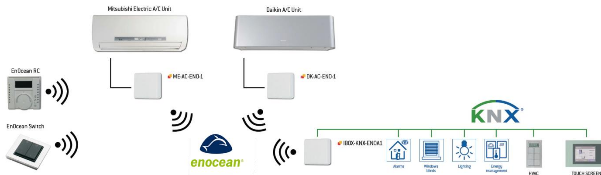
Figure 2.1 IBOX-KNX-ENO-A1 / A1C integration example
