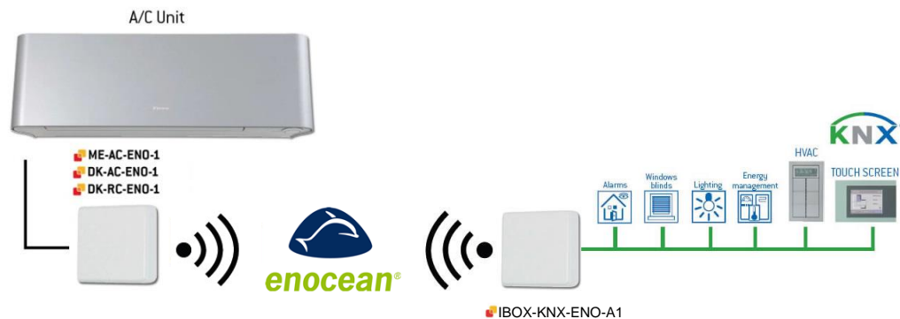
Figure 3.1 IBOX-KNX-ENO-A1 / A1C and IntesisBox Air Conditioner integration example
