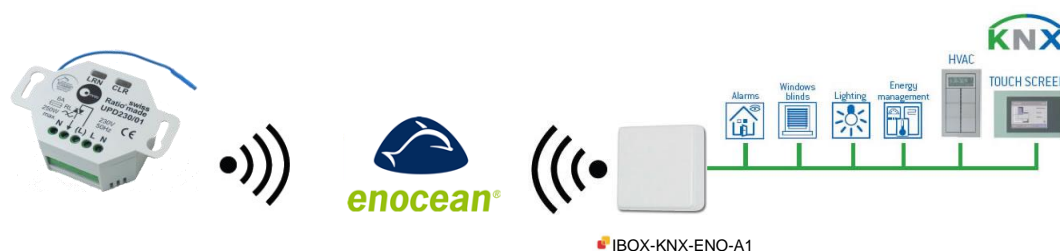
Figure 3.2 IBOX-KNX-ENO-A1 / A1C and light actuator integration example
