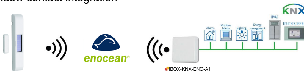
Figure 3.3 IBOX-KNX-ENO-A1 / A1C and Window Contact integration example
