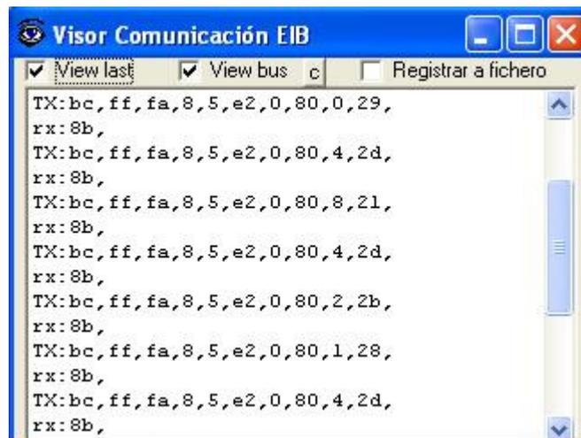
To monitor the communication between IntesisBox and the external system (*BACnet* in this case), select the menu *View -> Bus -> External system*. The *External protocol communication viewer* window will be opened. This window shows in real time all the communication frames between IntesisBox and the BACnet devices as well as debugging messages referent to external protocol (BACnet) sent by IntesisBox.
