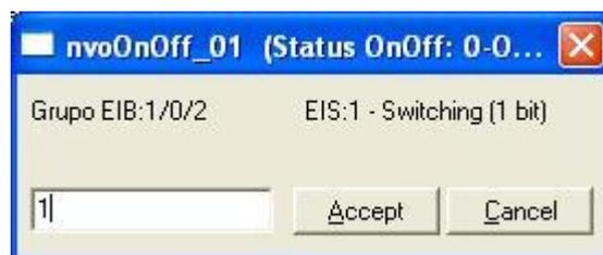
This tool is very useful to test any of the systems connected to the IntesisBox, KNX and LON without the need to actuate on the real signals.
