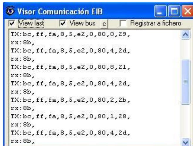
To monitor the communication between IntesisBox and the external system (*LON* in this case), select the menu *View -> Bus -> External system*. The *External protocol communication viewer* window will be opened. This window shows in real time all the communication frames between IntesisBox and the LON devices as well as debugging messages referent to external protocol (LON) sent by IntesisBox.
