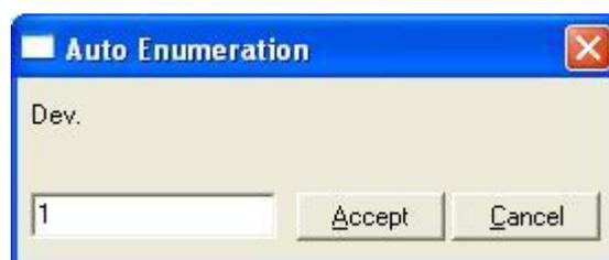
4. Enter the increment between consecutive assignments. For example selecting 0 for the first value and an increment of 1, the values generated will be 0,1,2,3,4.. and so on. To assign the same value to all the rows (useful to assign the same Device number in the column *Dev* for some consecutive rows) just select the desired value and an increment of 0.
