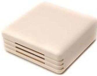
ME-AC-ENO-1 and ME-AC-ENO-1C devices allow a complete and natural integration of Mitsubishi Electric air conditioners with EnOcean control systems both in their 868 MHz (ME-AC-ENO-1) and 315 MHz (ME-AC-ENO-1C) versions.
