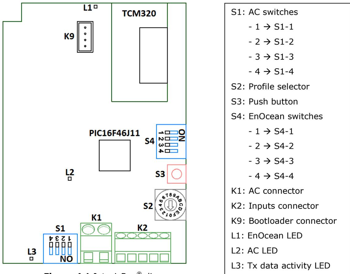
Figure 4.1 IntesisBox® diagram
