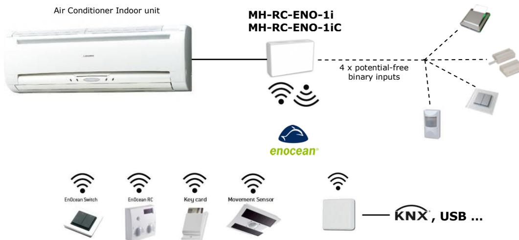
IntesisBox<sup>®</sup> MH-RC-ENO-1i / 1iC (IntesisBox<sup>®</sup> from now on) allows monitoring and control, fully bi-directionally, all the functioning parameters of Mitsubishi Heavy Industries air conditioners from EnOcean installations.
