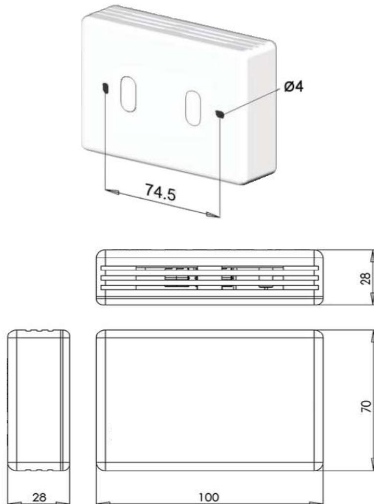
**Figure 10.1** IntesisBox<sup>®</sup> dimensions in mm
