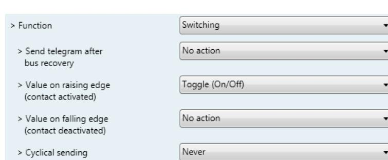
**Figure 4.42** Parameter detail
