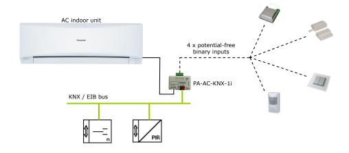
IntesisBox® PA-AC-KNX-1i allows monitoring and control, fully bi-directionally, all the functioning parameters of PANASONIC Air Conditioners from KNX installations. Compatible with all the models of the Etherea MKE line commercialised by PANASONIC.
