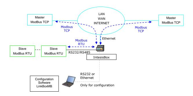
Transparent operation: the ModBus TCP telegrams are converted to ModBus RTU and vice-versa transparently.
