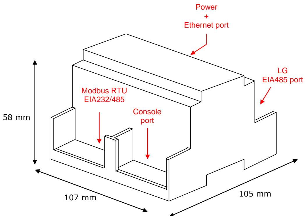
Recommended available space for its installation into a cabinet (wall or DIN rail mounting), with space enough for external connections:
