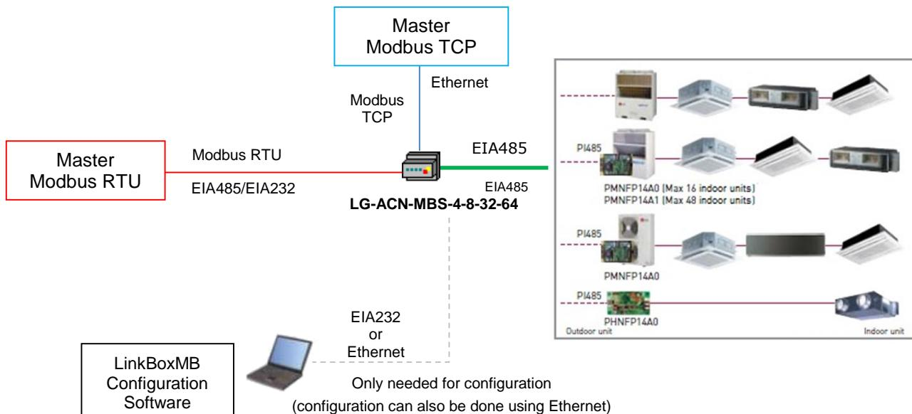
This integration requires the LG AC system being equipped with the LG PI485 interface or the proper connector in the Outdoor Units. There are four models available: LG-AC-MBS-4, with capacity of up to 4 indoor units, LG-AC-MBS-8, with capacity of up to 8 indoor units, LG-AC-MBS-16, with capacity of up to 16 indoor units and LG-AC-MBS-64, with capacity of up to 64 indoor units. Contact your nearest LG AC Systems distributor for details. More details about the PI485 interface and the AC specs.
