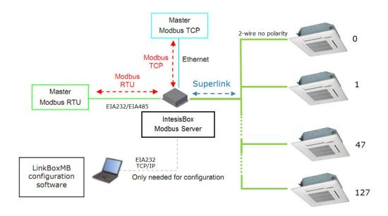
This gateway allows integrating a Mitsubishi Heavy Industries AC system inside a supervision/control/automation system through PLC, SCADA and, in general, through any device or system with Modbus mastering (TCP or RTU) interface.
