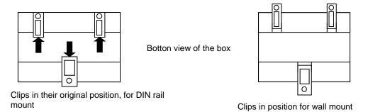
2. Use the holes of the clips to fix the box in the wall using screws. Use the template below for the wall holes.
