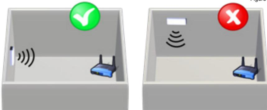
Antenna in vertical position and pointing to the Wi-Fi Access Point or Router.
