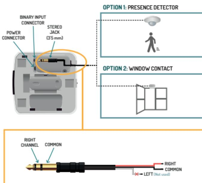
[EN] Connection cable not provided. Check requirements below.
