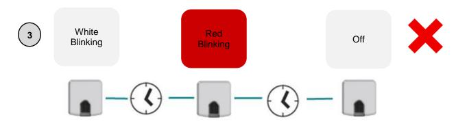
Note: The red blink means that the IR command has not been correctly recognized and therefore indicates that the remote controller used is not included in the device database. In this case, try it again and if the result is similar, contact with our support department.
