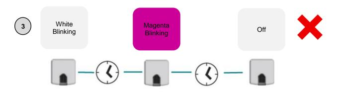
Note: The magenta blink means that the device is not connected to the internet. Please, check if the device is correctly connected to the available WiFi network and if the network has internet connection.
