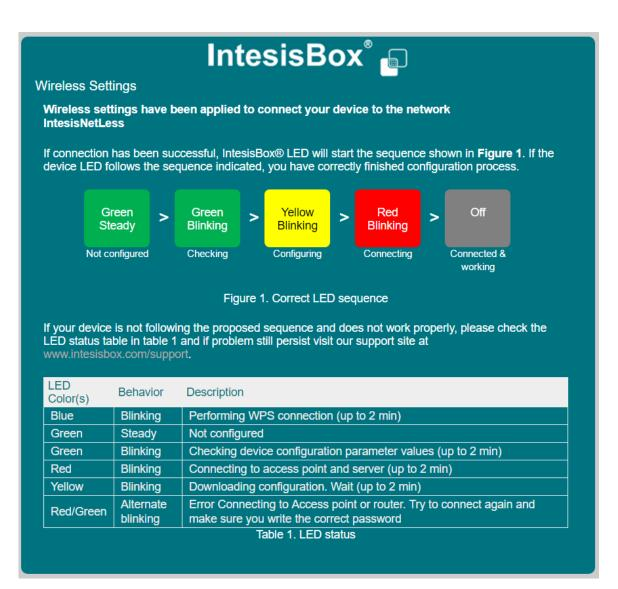
Once the WiFi configuration is completed, the product will save it and, under normal conditions, it is not necessary to do it again. Only in case the router is replaced on the network or the SSID or password are modified, the network configuration process needs to be redone. For this, it is necessary to restart the product back to factory mode (access point) by pressing the device button during 10 seconds. The LED will take the colour green if the factory mode has been acquired successfully.
