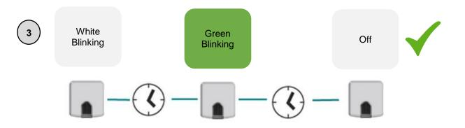
Note: The green blink means that the IR command has been correctly recognized and that the WMP product has been configured with the corresponding remote model. Therefore, the green color indicates that the process has finished successfully.
