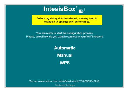
Note: in order to connect to the product properly, it is important to be only connected to the product WiFi network. If the PC or mobile has internet connection, it must be deactivated (disconnect ethernet cable, disconnect other WiFi connections, deactivate 3G...).
