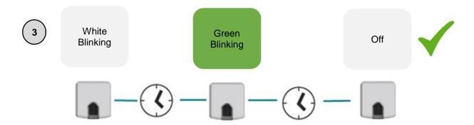
Note: The green blink means that the IR command has been correctly recognized and that the WMP product has been configured with the corresponding remote model. Therefore, the green color indicates that the process has finished successfully.
