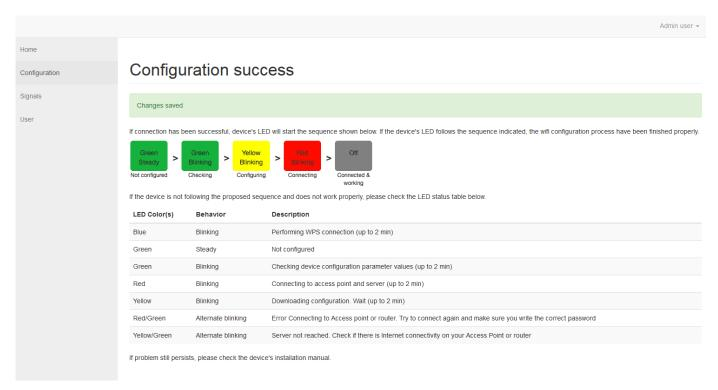
If process finishes and LED is not off (Red/Green or Yellow/Green blinking), it's possible that reconfiguration of the device is needed (for example, if wrong password for Wi-Fi was entered, etc).
