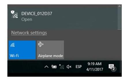
Connect your PC or mobile to this network and use the following web page/IP to connect the WiFi device to the WiFi network: **192.168.10.1.**
