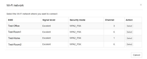
Desired Wi-Fi network / Access point must be selected (button **Select**). This will move the SSID to corresponding field of previous section (Access Point settings), where corresponding password for the SSID/Wi-Fi network must be entered.
