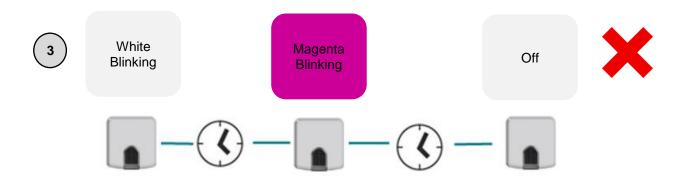
Note: The magenta blink means that the device is not connected to the internet. Please, check if the device is correctly connected to the available WiFi network and if the network has internet connection.
