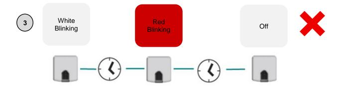
Note: The red blink means that the IR command has not been correctly recognized and therefore indicates that the remote controller used is not included in the device database. In this case, try it again and if the result is similar, contact with our support department.
