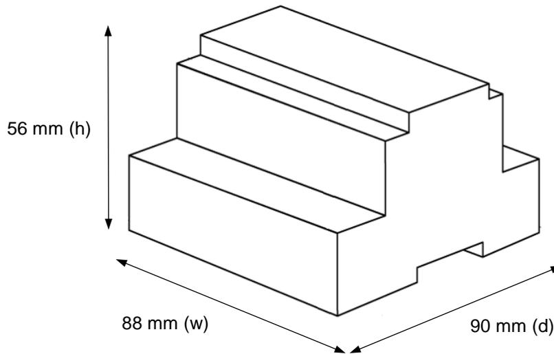
Recommended available space for its installation into a cabinet (wall or DIN rail mounting), with space enough for external connections
