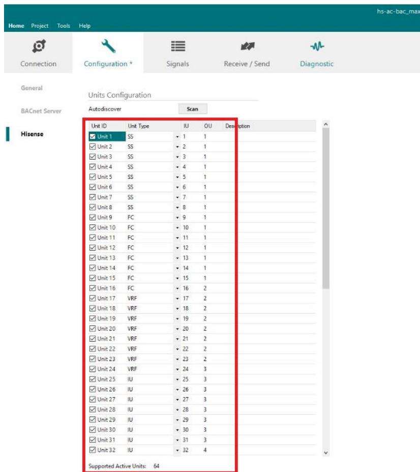
Figure 4.7 IntesisBox MAPS Hisense configuration tab after importing scan results
