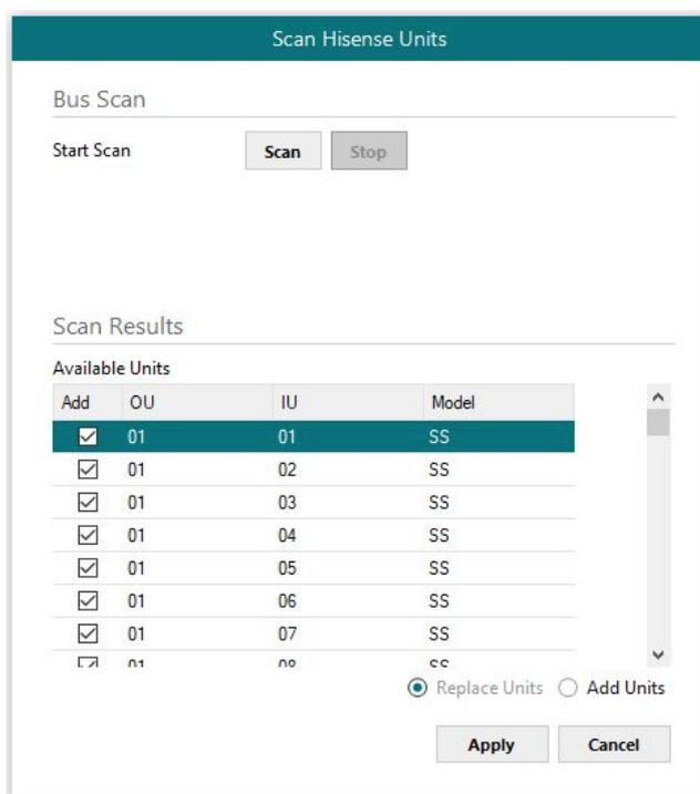
Figure 4.6 IntesisBox MAPS Scan Hisense Units window with scan results
