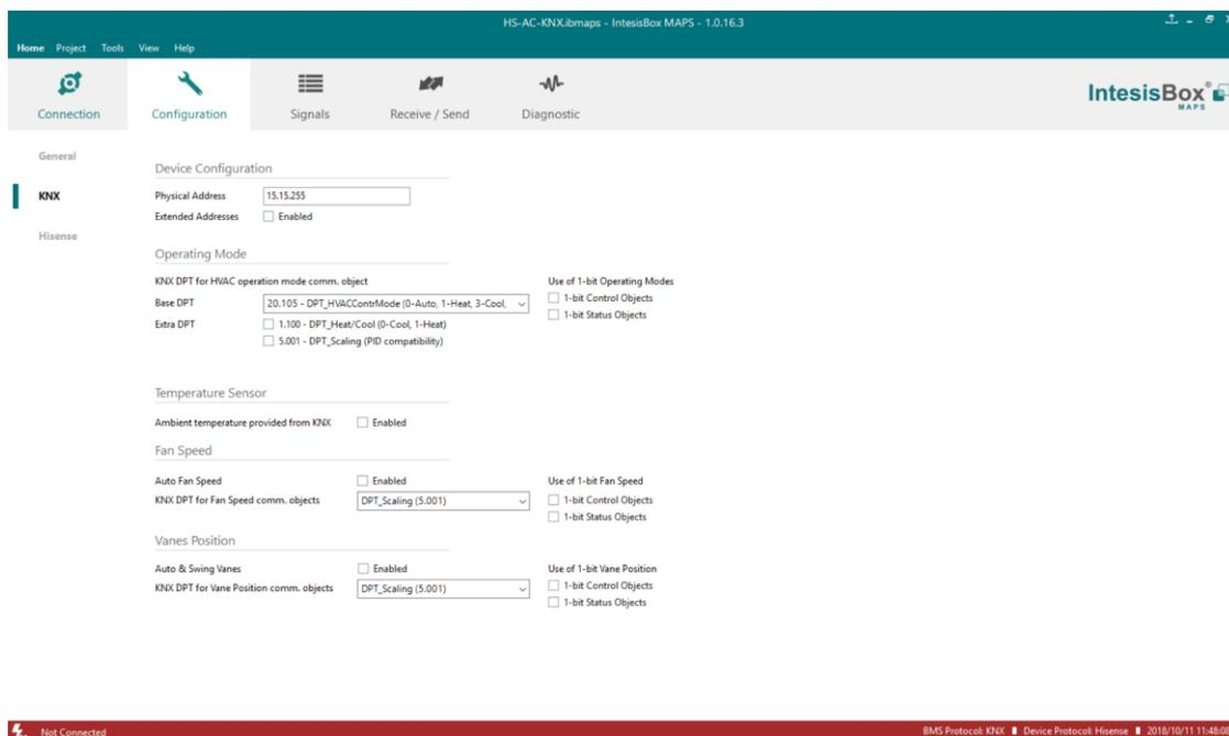
Figure 4.3 IntesisBox MAPS KNX configuration tab
