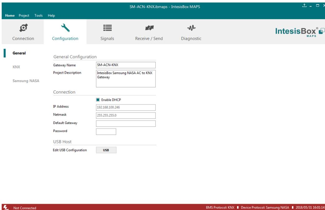
Figure 4.2 IntesisBox MAPS configuration tab
