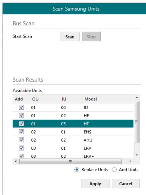
Figure 4.6 IntesisBox MAPS Scan Samsung Units window with scan results
