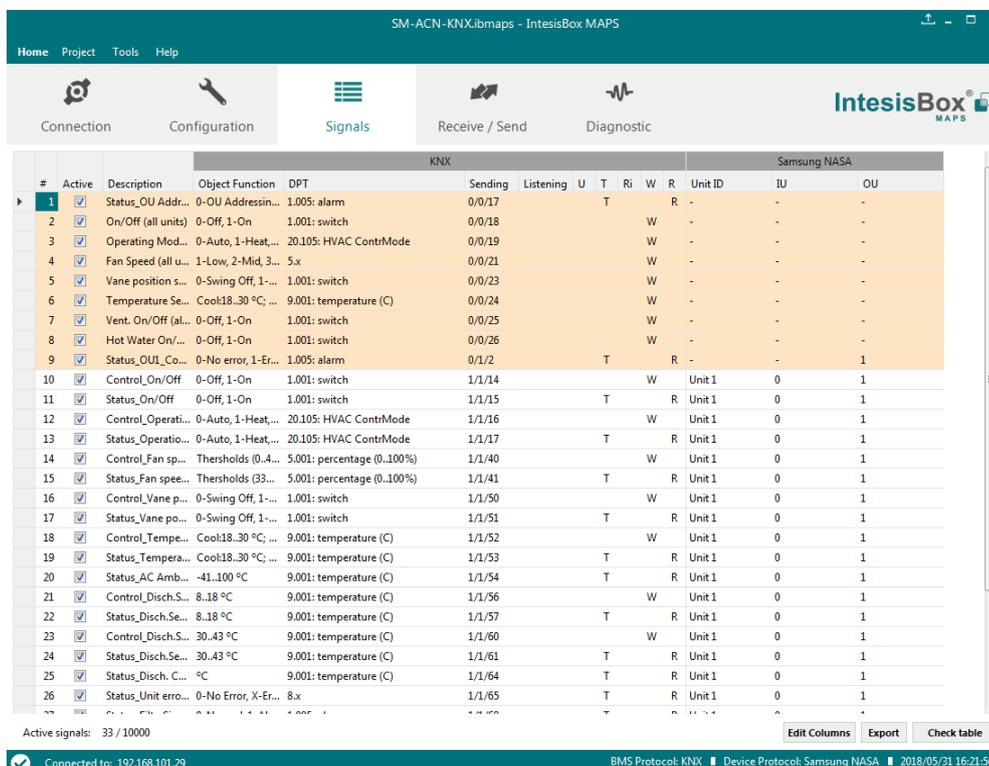
Figure 4.8 IntesisBox MAPS Signals tab
