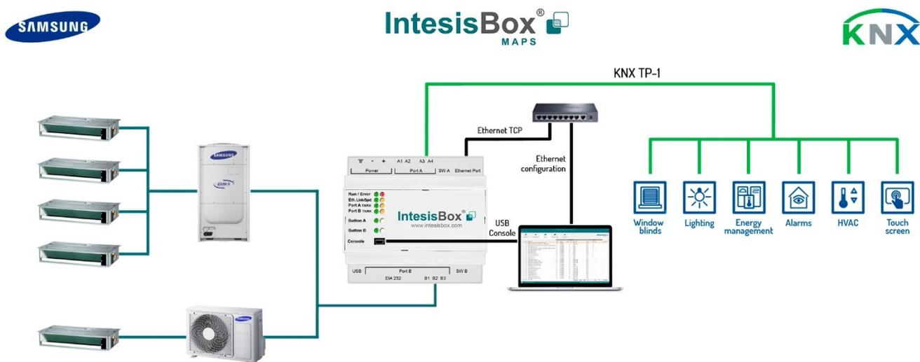
Integration of Samsung NASA's compatible systems into KNX home automation systems
