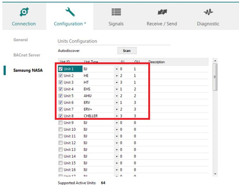
Figure 4.7 IntesisBox MAPS Samsung NASA configuration tab after importing scan results
