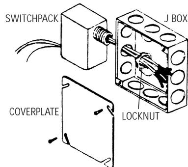
**CAUTION:** Do not run the sensor wire in the same conduit as power conductors. Install in accordance with local codes.
