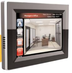
Th**E CLCTSIX** is a 7-inch diagonal, high resolution, wide-screen format, color LCD used for interfacing with the LightSweep<sup>™</sup> modular lighting control system. The CLCTSix uses BACnet over Ethernet to communicate with controllers on a local area network. User created graphics allow the CLCTSIx to be completely customized for a given application.
