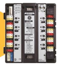
The **CLCGSM8** Group Switch Module will connect up to eight inputs to the Modular Lighting Control System. Through the color-coded spring clip terminals, the device supports switches, photocells and motion sensors. When not used for switches, the pilot light terminals may be configured to provide power to the connected sensors simplifying installation.
