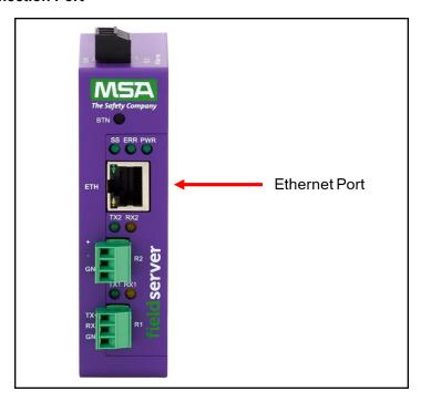
The Ethernet Port is used both for BACnet/IP communications and for configuring the gateway via the Web App. To connect the gateway, either connect the PC to the Router's Ethernet port or connect the Router and PC to an Ethernet switch. Use Cat-5 cables for the connection.
