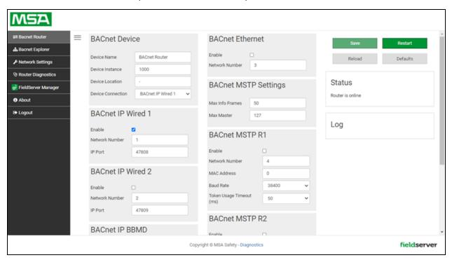
NOTE: For BACnet/IP, click on the Connections tab to ensure the gateway is on the BACnet/IP network subnet or to configure BBMD.
