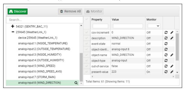
A full list of the device details will appear on the right side window. If changes are expected since the last explore, simply press the Refresh button (  $\mathfrak{Z}$  ) that appears to right of individual properties to refresh.
