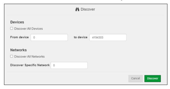
NOTE: The "Discover All Devices" or "Discover All Networks" checkboxes must be unchecked to search for a specific device range or network.
