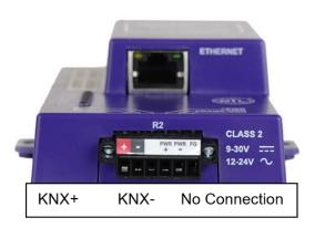
The KNX Connector consist of a KNX + and KNX- terminal. Each terminal corresponds to the red KNX+ and gray KNX- bus connections on a KNX bus.
