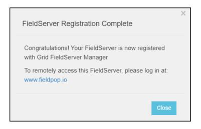
• Once the device has successfully been registered, a confirmation window will appear. Click the Close button and the following screen will appear listing the device details and additional information auto-populated by the QuickServer.
