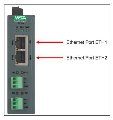
The Ethernet Port is used both for BACnet/IP communications and for configuring the gateway via the Web App. To connect the gateway, either connect the PC to the Router's Ethernet port or connect the Router and PC to an Ethernet switch. Use Cat-5 cables for the connection.
