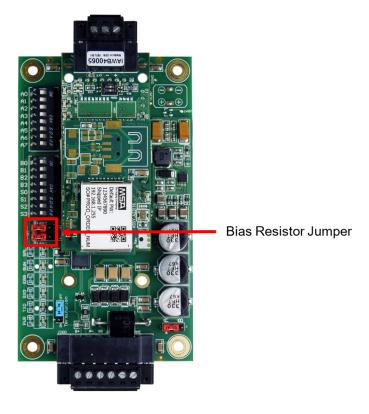
The QuickServer bias resistors are used to keep the RS-485 bus to a known state, when there is no transmission on the line (bus is idling), to help prevent false bits of data from being detected. The bias resistors typically pull one line high and the other low - far away from the decision point of the logic.
