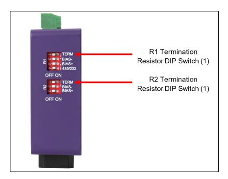
If the gateway is the last device on the serial trunk, then the End-Of-Line Termination Switch needs to be enabled. **To** enable the Termination Resistor, move the TERM dip switch to the right in the orientation shown in above.
