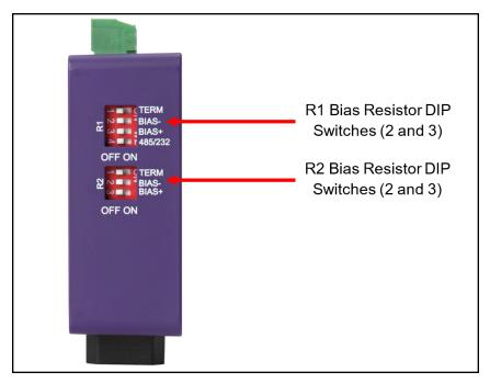
To enable Bias Resistors, move both the BIAS- and BIAS+ dip switches to the right in the orientation shown above.
