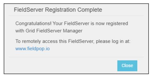
• Once the device has successfully been registered, a confirmation window will appear. Click the Close button and the following screen will appear listing the device details and additional information auto-populated by the QuickServer.
