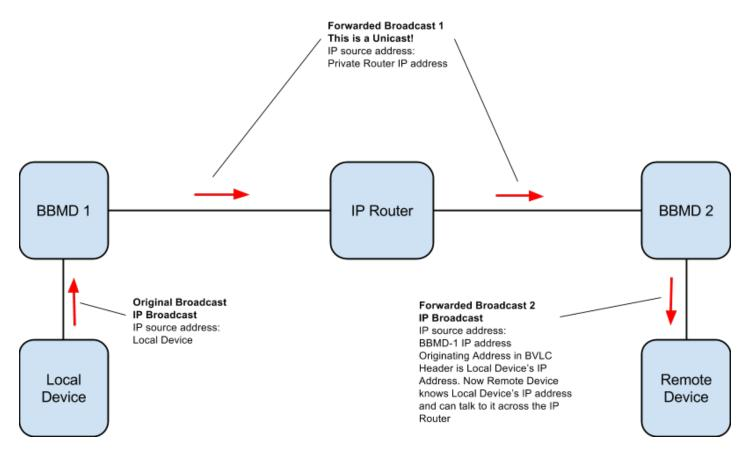
With NAT Routing, BBMD alone does not work because the Devices cannot reach each other's IP Addresses even if they know them. The only reachable address is the BBMD itself, so this must also act as a BACnet IoT Gateway to forward traffic to the intended device. When this is done, the destination device's IP Address and Port are encoded as the DADR in the network header, so that the Router can forward messages to the correct device.
