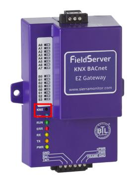
The KNX Administrator will request that the installer hit the service pin at the correct step of the commissioning process. Insert a small screwdriver or other device into the KNX port to activate the service pin when prompted.
