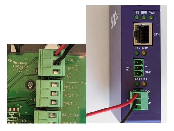
RS485 is meant to be carried on a twisted pair with a drain wire connected to the shiel.
