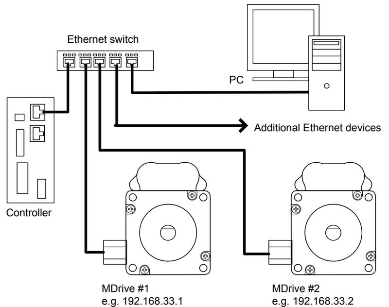
Figure 1.1: Example TCP/IP network with MDrive products.
