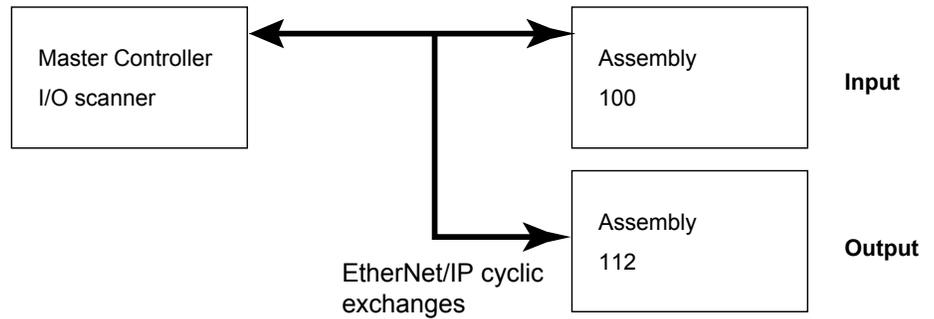
Figure 3.1: Overview of communication means
