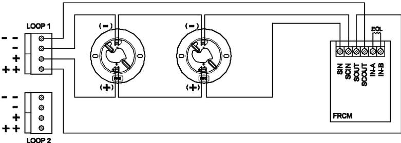
Complete loop wiring. Installation of sensor bases at this time is acceptable. If using a high voltage testing device to verify ground isolation, do not expose devices or modules to the high voltage.
