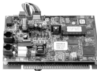
MDACT → Multi-Point Digital Alarm Communicator Transmitter
