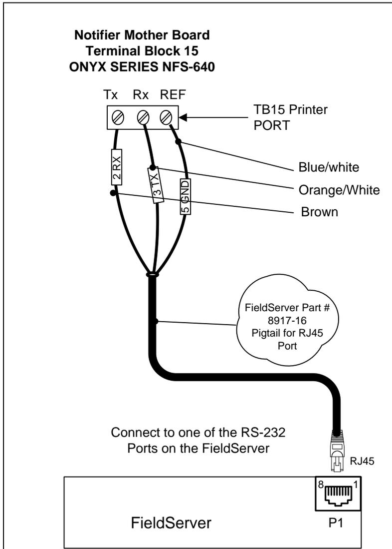
The FieldServer is connected to the Notifier Onyx NFS2-640 Panel as shown below. Configure the Notifier Onyx NFS2-640 Panel according to manufacturer's instructions. Note that the recommended connection through the printer port is depicted in the diagram. If preferred, connection can be made through the CRT port. Refer to Appendix A.4.3 for more information.
