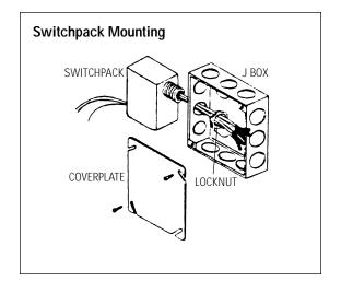
CAUTION: Do not run the sensor wire in the same conduit as power conductors. Install in accordance with local codes.
